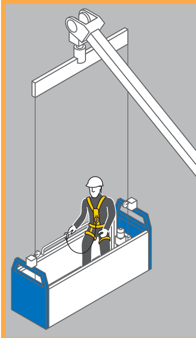
FIGURE 15: An example of a building maintenance unit with safety harness and restraint line.
