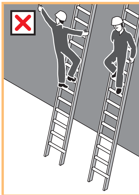
Facing away from the ladder to descend; over-reaching
