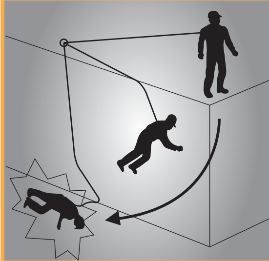
FIGURE 23: During 'swing down' the length of the lanyard and positioning of the anchor allow contact with the ground.
